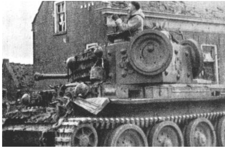
“Cromwell” tank at listening post near the river Maas embankment. Note the two track wheels and track parts on the tank’s turret and in front of the tank. Both items were welded on and were supposed to deflect armor piercing shells. Opposite is the building where the cat played with the billiard balls.
